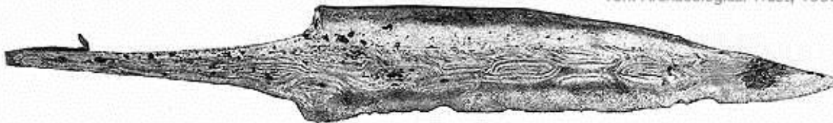
b After final descaling. The slight etching effect shows the darker steel cutting edge, the steel components of the pattern welding, and the steel 'sealing strip' along the knife back. Note the ductile folding of the cutting edge
